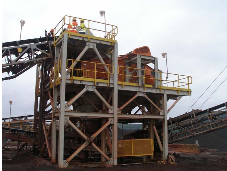
Exhibit 7: Primary and secondary wet screens
