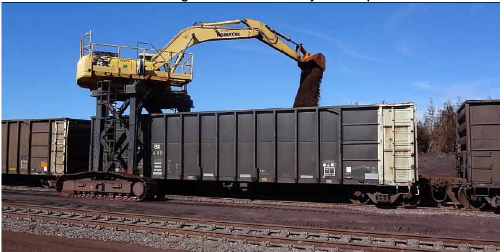
Exhibit 153: Excavator unloading a train at IOC's stockyard at Sept Iles
