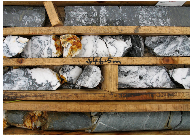
Figure 4. Near-massive sulfides in top slot overlain (downhole) by quartz-rock (slots 2 and 3), then chloritized rhyolite B (slot 4). Assay at 44.75-45.70m: 0.95m at 1.47 % Cu, 14.13 % Pb, 25.52 % Zn, 115 g/t Ag and 2.99 g/t Au.
