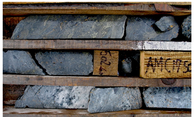
Figure 5. Massive sulfides (top slot) overlying silicified and sulfidized rhyolite B (slots 2 and 3). Garth Daniels area, hole AMC-17. Assay at 496.6-502.1m: 5.5m at 3.73 % Cu, 6.06 % Pb, 12.51 % Zn, 78 g/t Ag and 0.37 g/t Au.
